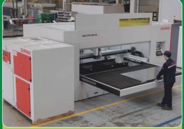
2 kW Fiber Lazer ile Çapaksız Kesim. Burr-free manufacturing via Laser Cutting Machine with 2 kW.
